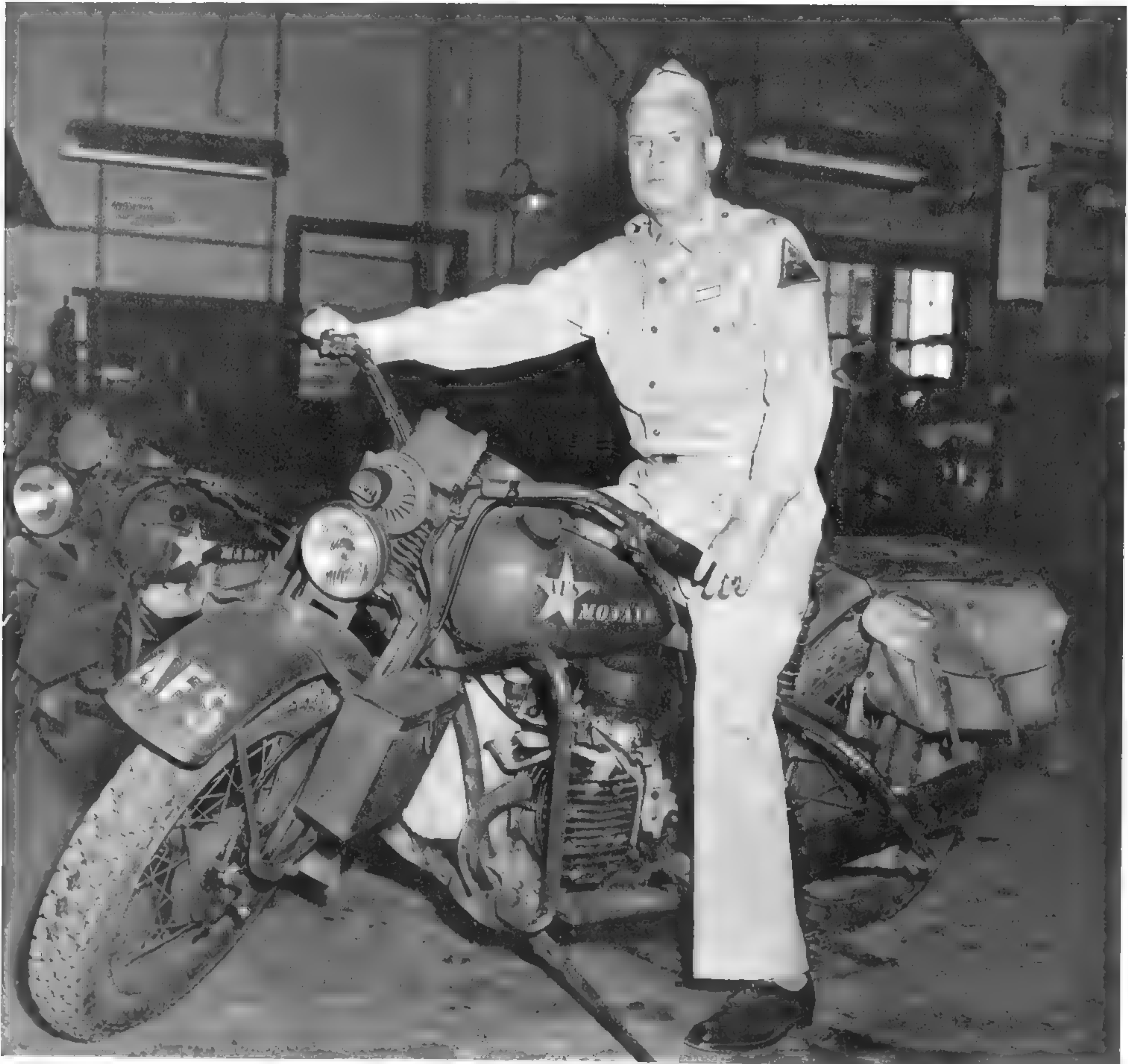
This Harley-Davidson XA was photographed during WWII at Ft. Knox, Kentucky. Lt. John E. Harley directed motorcycle training there in 1942. The head of the horizontally opposed engine is visible just ahead of the rider's leg. (Photo courtesy of the Patton Museum)
